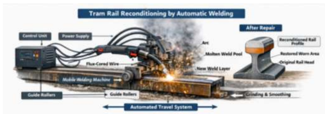
Figure 4. Tram rail reconditioning by automatic welding
