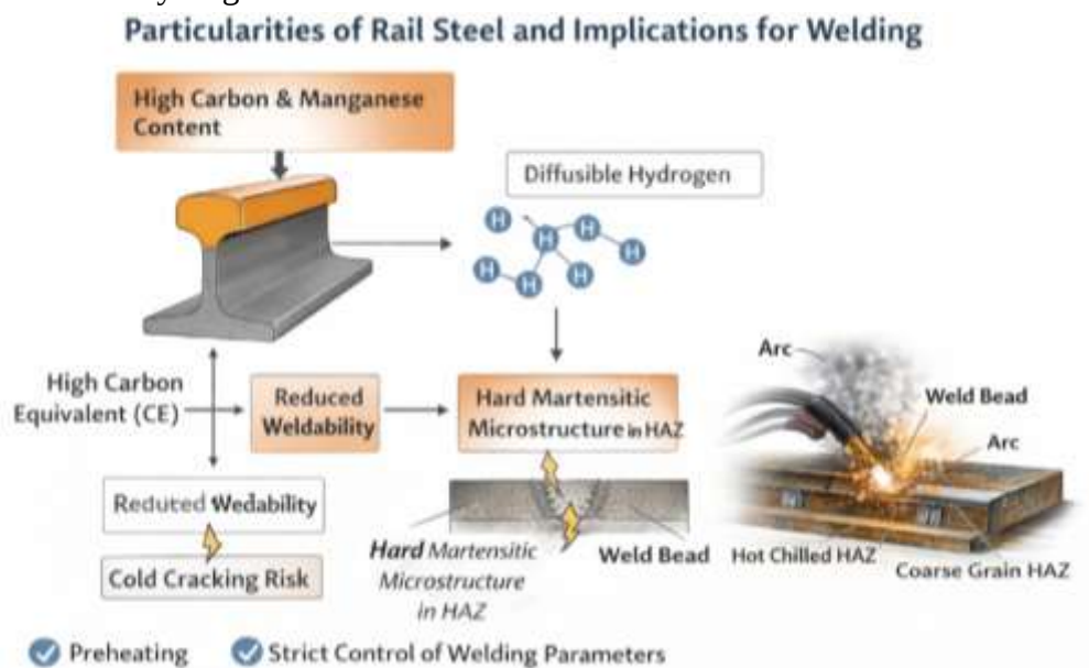
Figure 1. Particularities of rail steel and implications for welding
