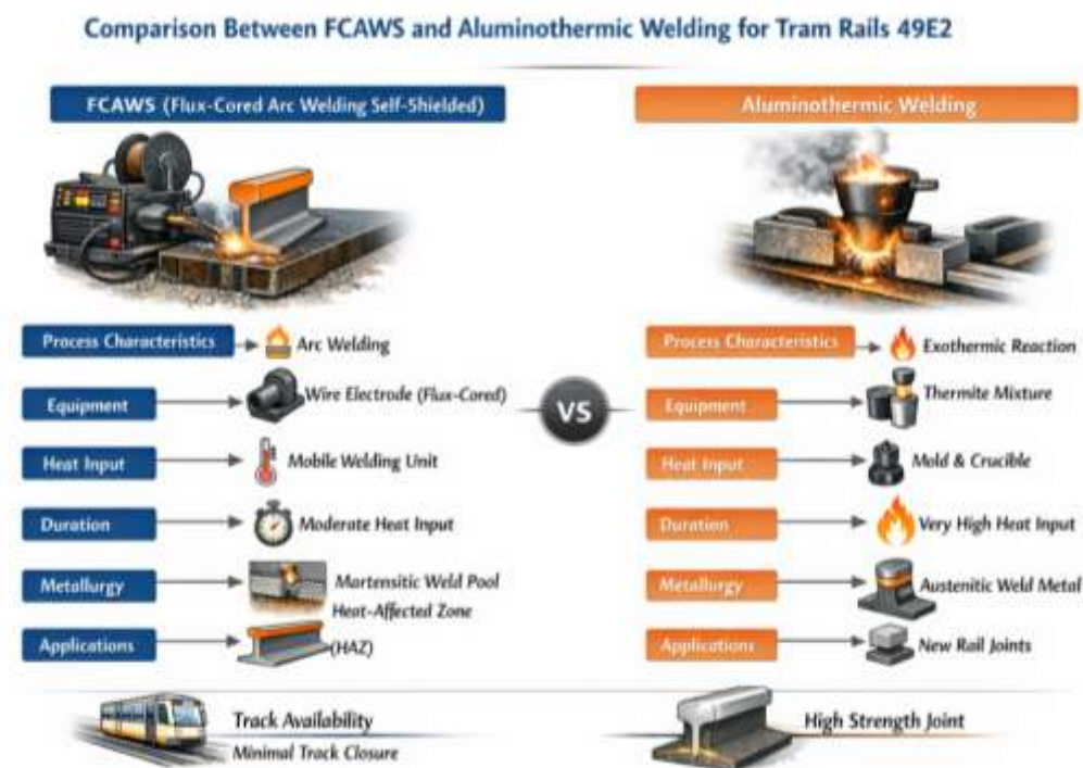
Figure 6. Comparison Between FCAWS and Aluminothermic Welding for Tram Rails 49E2
