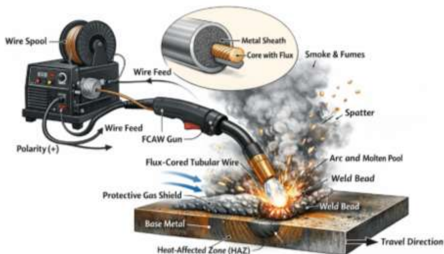
Figure 3. Self-Protection Tubular Wire Welding (FCAWS)
